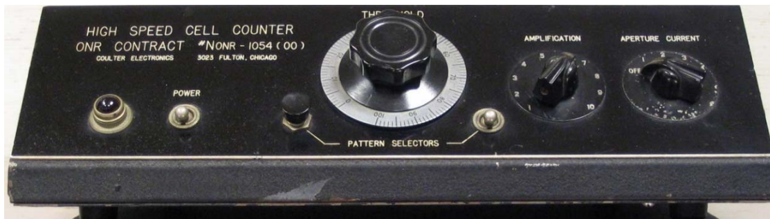
Figure 4.3. The electronics module from the initial ONR work. It integrated the voltage supply for aperture current and the amplifier for cellular pulses resulting when cells modulated the current as they transited the aperture. The first switch from the right controlled the current to the aperture, and the second one set the pulse amplification. The large center knob controlled the threshold, or level, above which the amplitude of a pulse had to be for it to be counted. Connectors for the aperture current, aperture signal, and an oscilloscope are on the module's rear panel. Photograph courtesy of William G. Graham.
