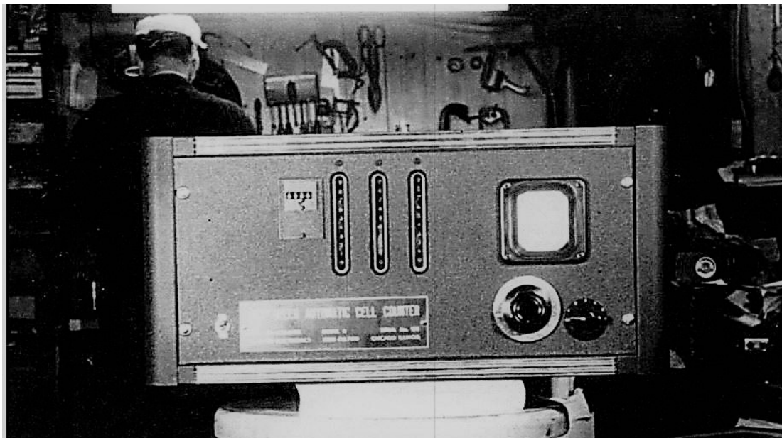
Figure 4.6. Electronics unit of a prototype Coulter Counter® Model A. The appearance differed from that of the first integrated and laboratory units via the panel label and the frame around the oscilloscope display being taller than it was wide. Wallace Coulter works behind the unfinished unit in the Coulter's W. Fulton basement; WHC Papers.
