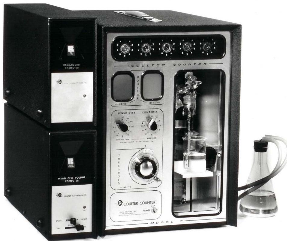
Figure 8.6. A Coulter Counter® Model F and accessory modules. 407 The first self-contained counter CEI developed, the transistorized Model F counter located the count display tubes at the technologist's eye level, with screens for monitoring the signal stream and the Coulter sensing aperture just beneath them. The latter received an image projected by an internal optical system focused on the sensing aperture, so eliminating the individual microscope used on the four earlier Coulter counters. 408 The digit counts were indicated by the position of a bright dot on the five dekatron tubes at the top of the panel. In addition to cell counts, the lower accessory module computed the mean cell volume (MCV) and from that result, the upper module computed the sample hematocrit (Hct). 409 Cell-volume distributions could be automatically plotted by the Model J plotter.
